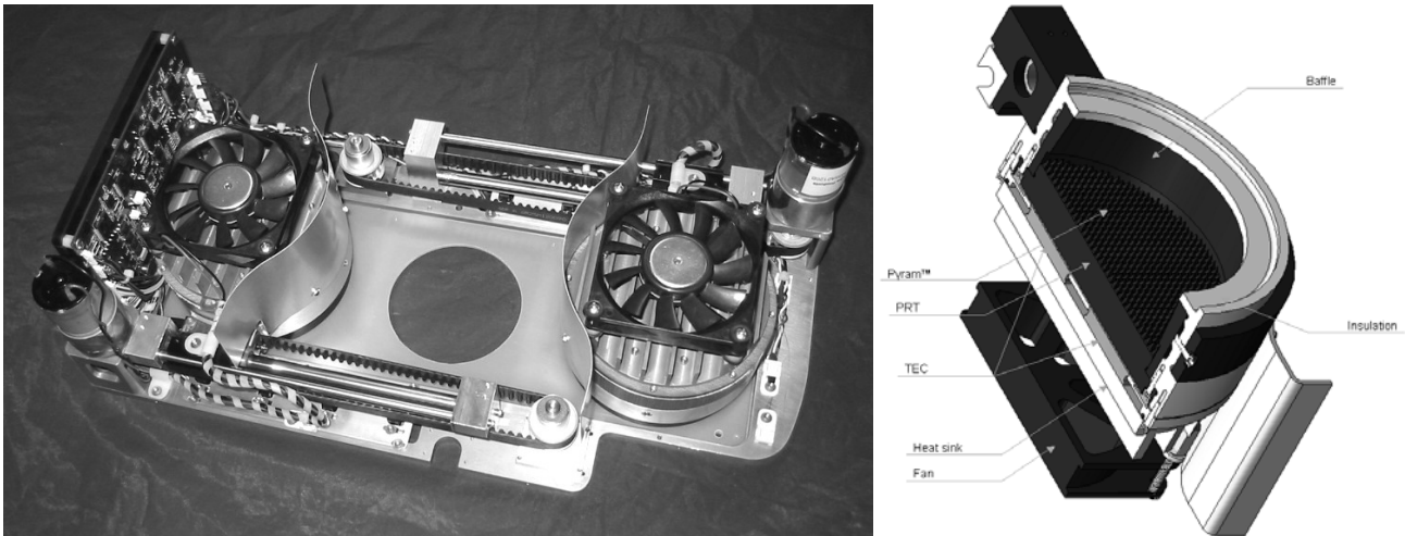
Fig. 6: Photograph of the calibration subsystem and cut view of a blackbody
