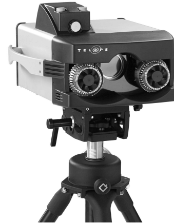
Figure 1: Picture of the FIRST, a LWIR hyperspectral imager
